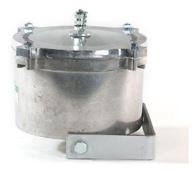
The Kleenoil filtration unit is made of cast aluminum with a stainless steel mounting bracket. It is connected to the engine lubricating oil circulating system in a bypass loop using high pressure braided hose and fittings to SAE standards.
